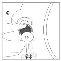
Remove transport safety bolts and rubber bushes by pulling outwards. (A up/down action and a small squirt of washing up liquid should ease
